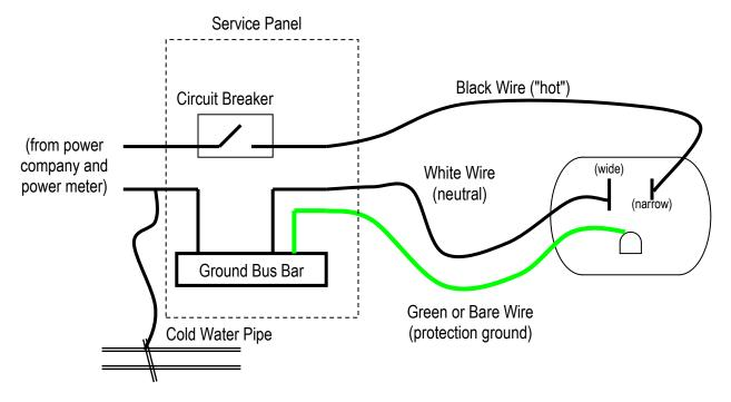
IF the outlet is wired correctly (never EVER risk your life on this assumption!!), the white wire ("neutral") should be the wide blade and the electrical potential should be near zero potential. In the U.S. the black wire ("hot") is 120 volts RMS (root-mean-square) sinusoid, 60 Hz repetition frequency, with peaks  $\pm 170$  volts respect to the neutral. Keep in mind that the colors are purely customary: the color itself doesn't influence how the electricity flows in the circuit.
