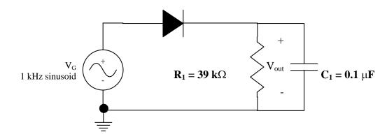
? Sketch (and LABEL) the waveform of the voltage across the resistor/capacitor combination, and indicate the maximum and minimum voltages that you measure.
