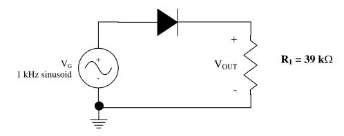
Set the input voltage amplitude to 2 V peak-to-peak and set the frequency to 1 kHz. Observe  $V_G$  on one channel of the oscilloscope and  $V_{OUT}$  on the other channel. Both channels should be set for <u>DC</u> <u>Coupling</u> in order to give proper readings.
