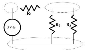
A *loop* is a connected path through a sequence of elements that starts and ends at the same node without crossing itself. A circuit must have at least one loop. If there is more than a single loop, the separate loops of a circuit generally partially overlap one another.
