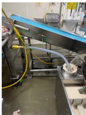
Cure recycle system captures wasted cure for re-use.
