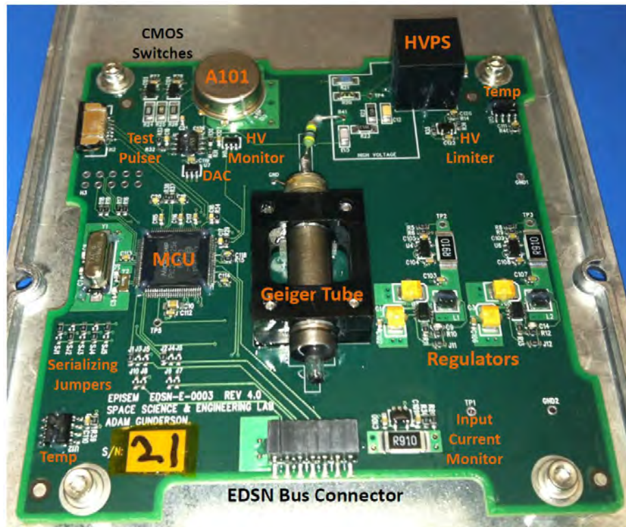
Figure 2.3: Image of the EPISEM circuit board displaying the location of the primary circuits and components. [16]
