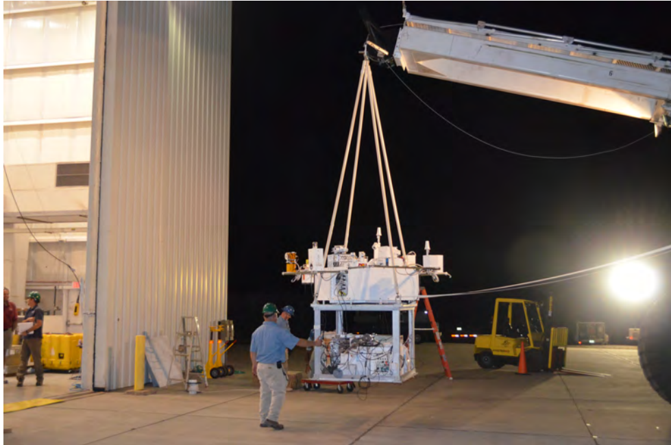
Figure 2.20: This figure shows the 2012 MSU HASP payload mounted to the HASP platform, which is suspended from the launch vehicle during the early stages of flight operations.
