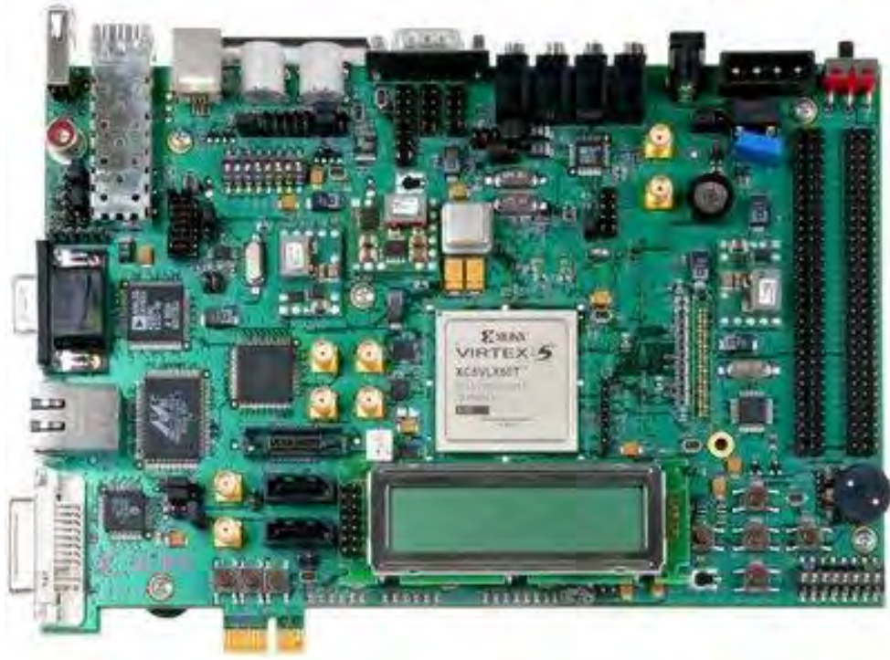
Figure 2.3: This figure shows the ML505 development board used for the implementation of many TMR+Spares w/Repair systems. The board features a Xilinx Virtex-5 FPGA.
