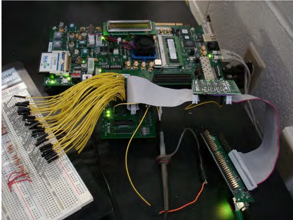
Figure 2.7: This figure shows the early hardware setup used in this research. It includes the ML605 development board, a general-purpose interface board for receiving radiation sensor inputs and a parallel-to-USB adapter board for communication with a host computer [10].
