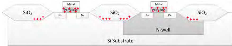
Figure 1.6: This figure shows the device cross-section for a CMOS circuit along with illustrations of TID-associated charge trapping in the gate and field oxides.
