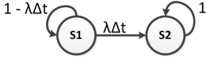
Figure 3.1: This figure shows the Markov chain for a simple, two-state system. The fault rate is given by \lambda . S1 is a healthy state and S1 is a failed state. \lambda\delta t is the probability of transitioning from S1 to S2 . As there is no recovery process, once the system reaches S2 it remains there with probability 1.
