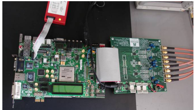
Figure 6. Xilinx ML507 board containing the Virtex-5 FX70 FPGA connected to a custom 12.5MSPS A/D.
